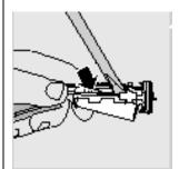
4. Insert the screwdriver under the circuit board, next to the battery connections, and twist to break the connections. Remove the circuit board and pry the battery from the plastic carrier.
