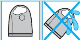
To prevent the cleaning fluid from leaking, ensure that the Clean&Renew station is placed on a flat surface. When a cleaning cartridge is installed, do not tip, move suddenly or transport the station in any way as cleaning fluid might spill out of the cartridge. Do not place the station inside a mirror cabinet, nor place it on a polished or lacquered surface.
