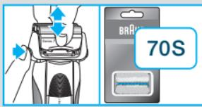
After you have replaced the Foil & Cutter cassette, use a ball-pen to push the reset button ⑯ for at least 3 seconds to reset the counter. While doing so, the replacement light blinks and goes off when the reset is complete. The manual reset can be done at any time.
